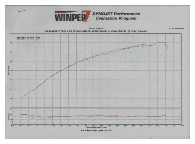
As can be seen from the chart, this Misano engine produces good power from 4,500 rpm up to 8,500 rpm. The broad spread of torque is ideal for the road as well as on–track.
