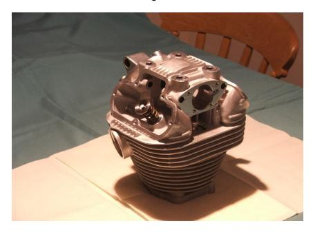
The ports and valve geometry have been optimised to allow far better performance than the original heads could achieve. All heads are supplied with two 10mm plug holes, the second plug situated to the rear of the bevel tunnel where the 450 decompressor plunger is fitted. The valve sizes are 41mm inlet, 34mm exhaust and both have 7mm diameter stems. The combustion chamber has an extensive continuous squish band which requires a modified piston.
