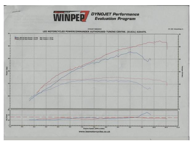
As can be seen from the dyno chart, this Misano engine produces good power from 6,000 rpm up to 10,500 rpm. The comparison shown is against the previous build of the same engine. This was an advanced Ducati Desmo specification developed by a very well respected tuner and owned by Nigel Palmer (UK Classic Racing 250 Champion).
